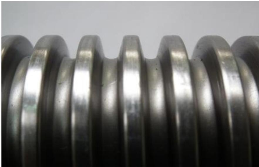
***Picture 4: Rolled thread – smooth surface***
