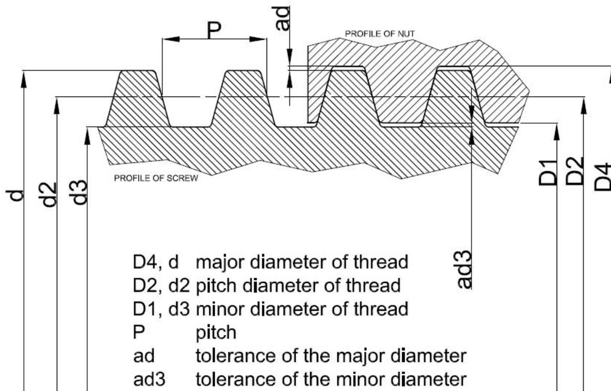
Picture 1: Sketch of a screw – nut, detail of thread
