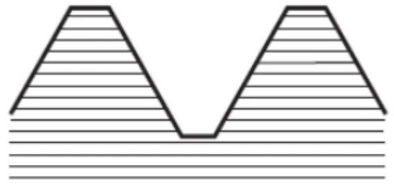
Picture 3: Machined thread
