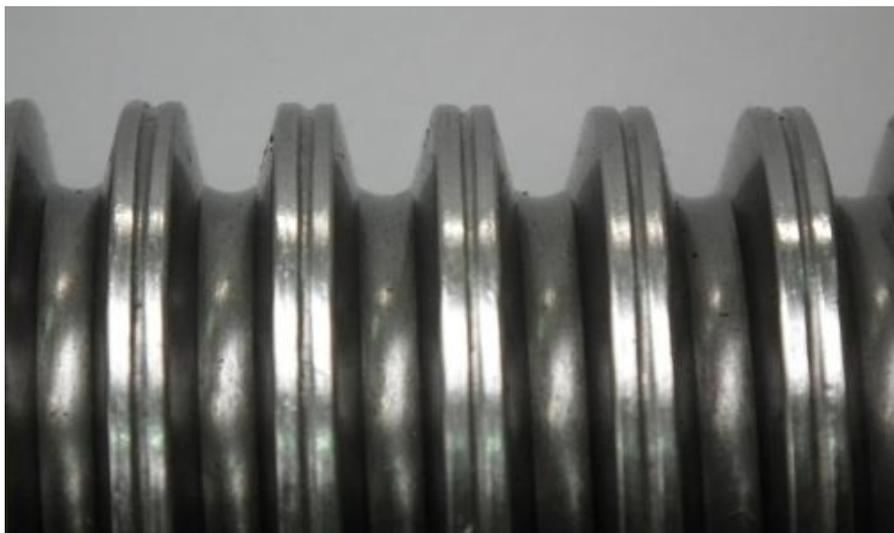
***Picture 5: Rolled thread with the groove on the outside surface***
