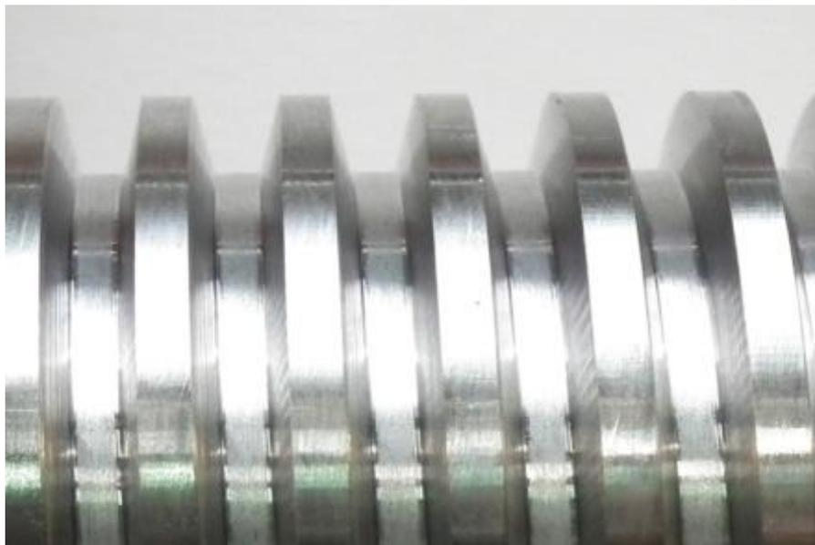
**Picture 6: Machined thread**
