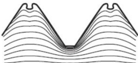
Picture 2: Rolled thread
